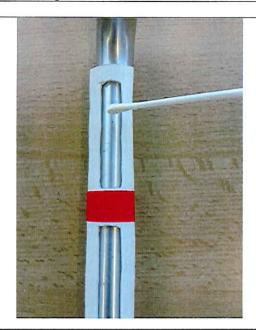
4. Example of swab being used within swab measuring apparatus
