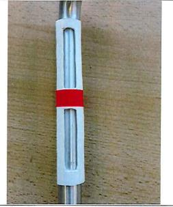
2. Swab area measuring apparatus affixed to rear of door handle [REAR VIEW]
