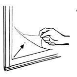
6. If a particle is trapped behind the film, carefully lift the film from the nearest corner and remove the particle. Before replacing the film, spray sufficient slip solution to thoroughly wet the glass and film. Replace the film and re-squeegee.
